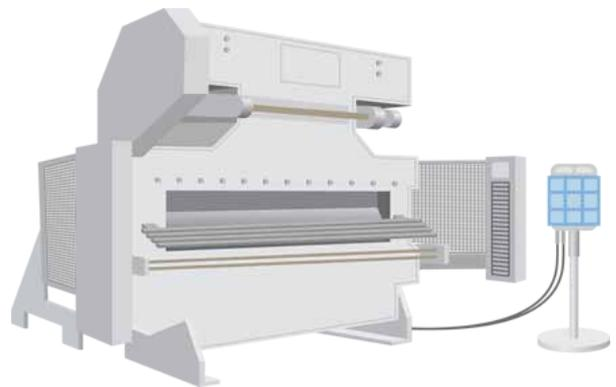
A photoelectric device fitted to a press brake; the device forms a curtain of beams across the front of the machine
