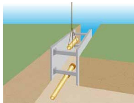
A trench box placed inside a trench creates a protected area for workers
