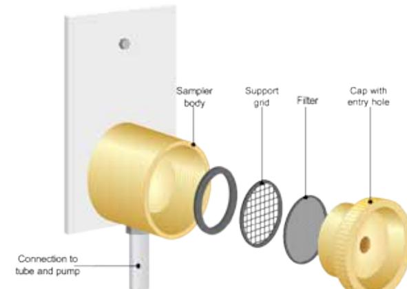
*Dust sampler head showing filter in position
