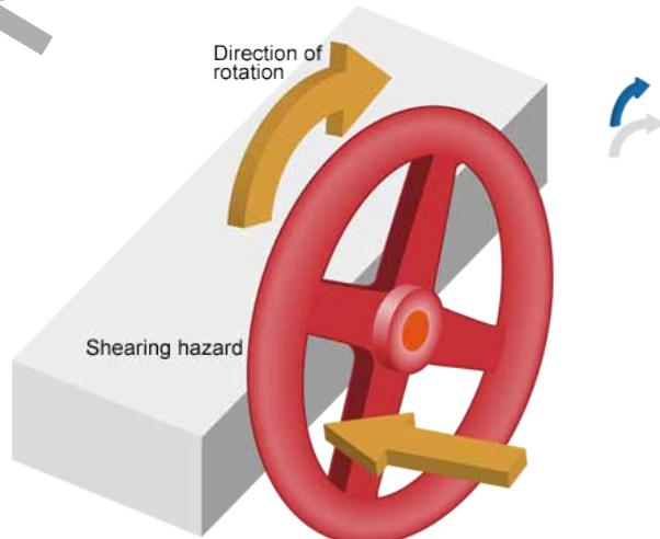
*Shearing – a finger put through the spokes of this wheel will be sheared off*
