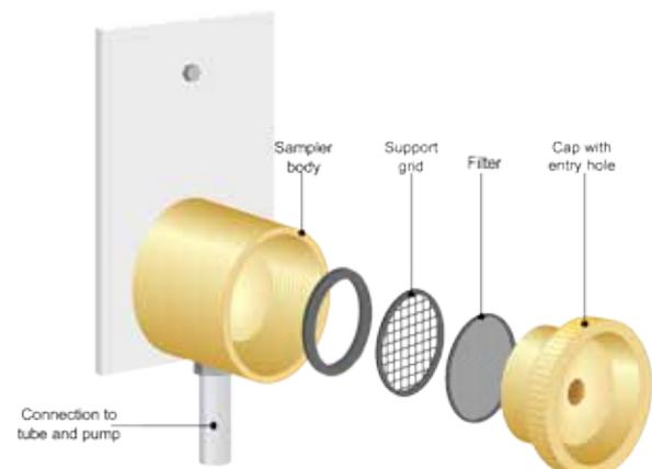
*Dust sampler head showing filter in position
